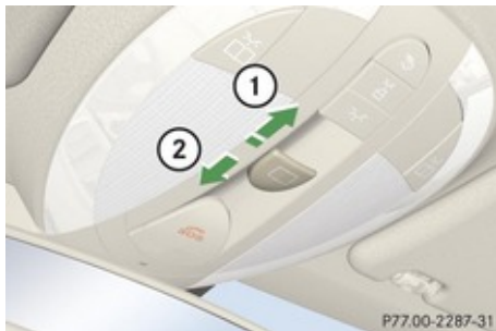
Roof panel switch
